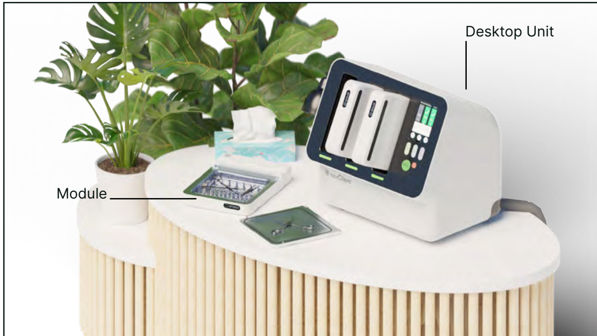
Figure 17. modClave: Desktop Unit and 3 modules with 1 unplugged.
