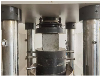
(a) Cube test block test instrument
