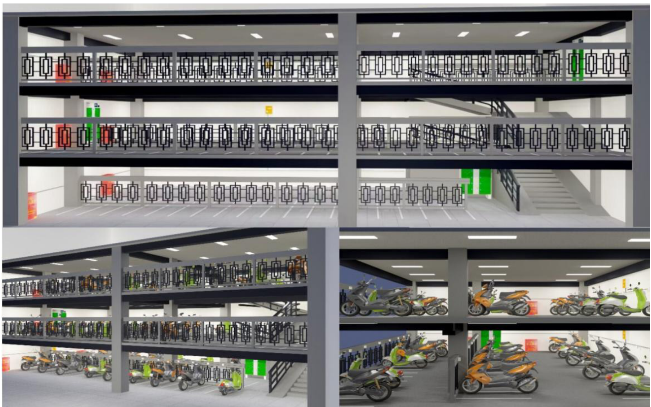
Figure 6. 3D design of multi-story assembled electric bicycle charging parking lot at multiple angles (Source: Design by Liya Fang)
