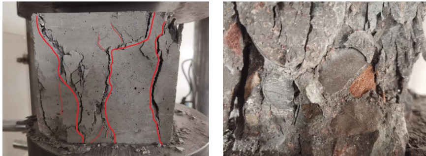
(c) Failure pattern of S80-0 test block
