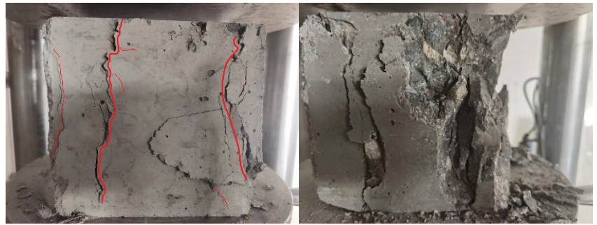
(b) Failure pattern of S60-0 test block
