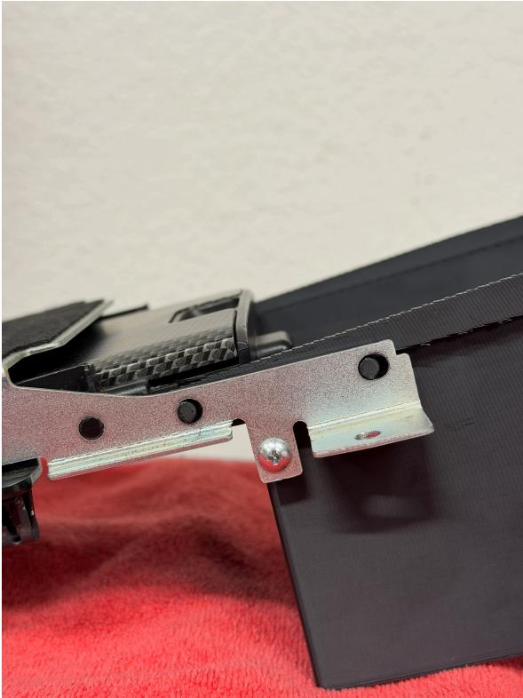
3. To remove the button, you'll have to remove the two pieces of foam tape that Honda installed on the sides. I circled where in red, however I didn't take pictures the first time I removed the button. Once the tape is removed, just slowly pull the button up, there's two tabs on the side of it that keep it in place. If yours is hard to remove, just use a hair dryer to make the plastic a bit more flexible. If you use a heat gun be mindful of the duration!
