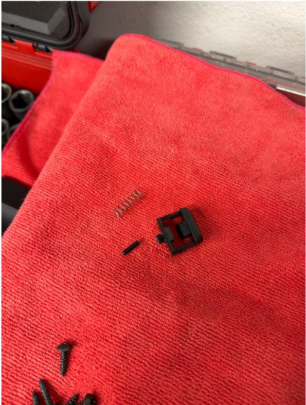
5. Place the spring over the spring retention hump and then press the button in! The tolerances are just perfect and there shouldn't be any binding.
