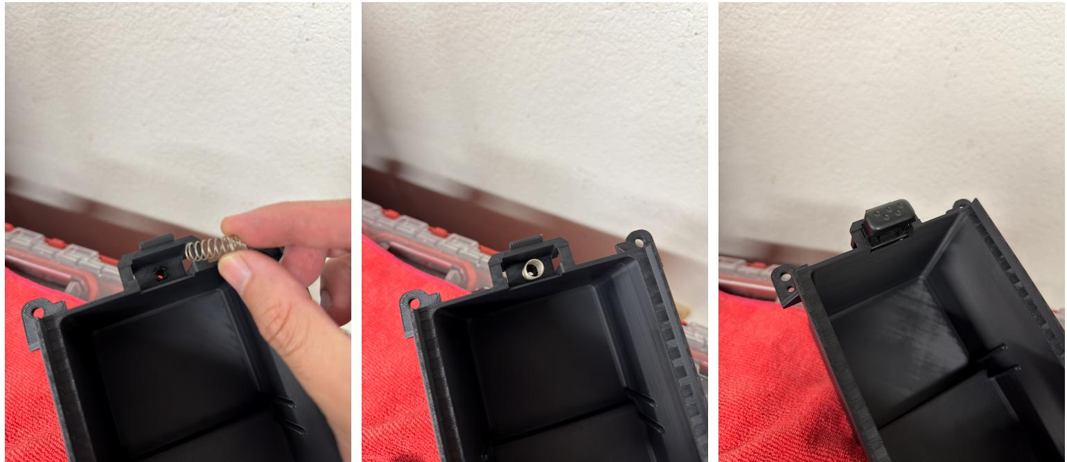
6. After this its just doing everything in the opposite order! One tip that I recommend, but not necessary, is to heat up the silver screws with a hair dryer or heat gun before screwing it in. Upon heating, it significantly helps with thread formation process. The mounting hole is engineered with increased mass surrounding the screw to ensure enhanced security and rigidity. Also take note of how the cup holder fits with the door assembly, it slots in just like OEM.
