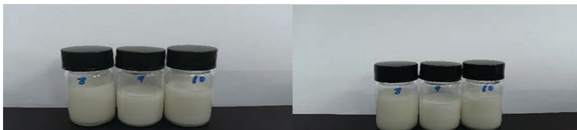
Figure 3. Appearance analysis diagram of emulsions with different homogeneous speed
