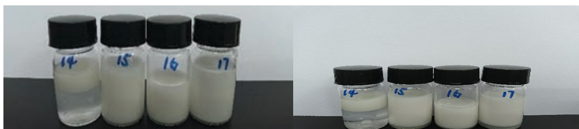
Figure 5. Appearance analysis of emulsions with different SA concentrations
