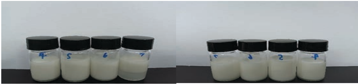
Figure 2. Appearance analysis diagram of emulsions with different aqueous phase proportions
