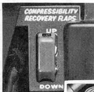
Figure 16— Compressibility Recovery Flap Switch
