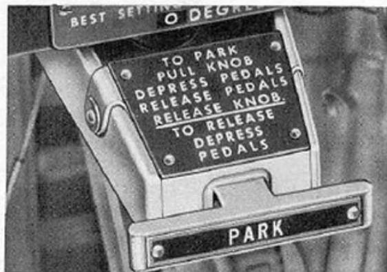
Figure 24—Parking Brake Control Through P-47D-28
