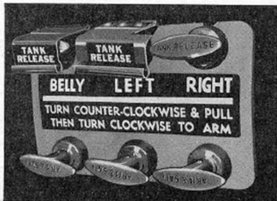
Figure 9—External Tank and Bomb Release Controls Through P-47D-27
