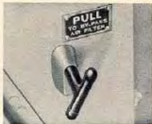
Figure 23— Air Filter Control
