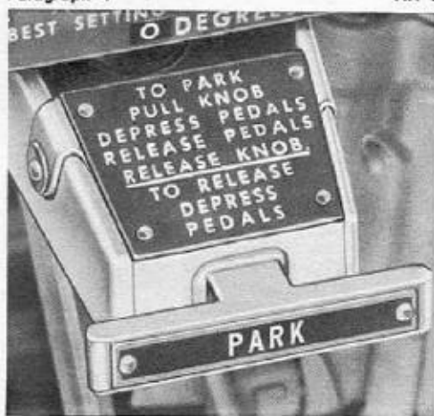
Figure 21—Parking Brake Control Handle
