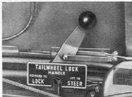
Figure 11—Tail Wheel Lock
