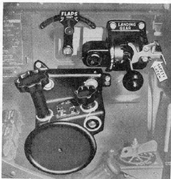
Figure 15—Trim Tab, Landing Gear, and Wing Flap Controls
