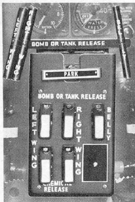
Figure 11—Electric Bomb Release Selector Panel P-47D-30 and Up
