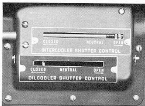
Figure 13—Oil Cooler and Intercooler Shutter-Position Indicators
