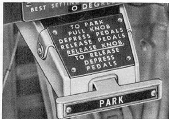
Figure 24—Parking Brake Control Through P-47D-28
